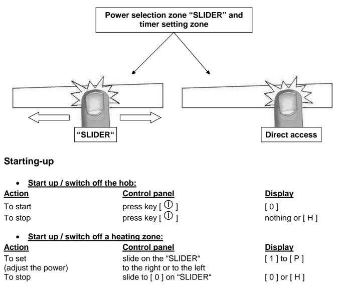
If no action is made within 20 second the electronics returns in waiting position.
