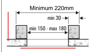
The minimum gap between your ceiling joist is 150mm.
